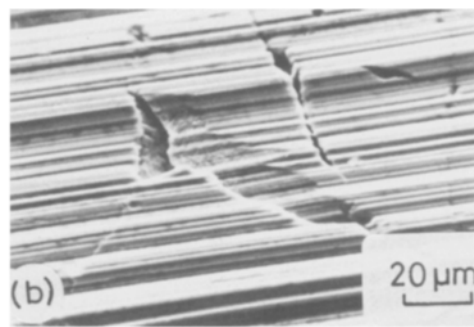
Figure 3 Scanning electron micrographs of surfaces of wear scars after sliding in 10 vol% acid-in-oil mixture (acid of 10% concentration) for 24 h. Disc specimens of 400 grit surface finish. (a) Pin specimen, applied load 2.5 kg; (b) pin specimen, applied load 4.0 kg; (c) disc specimen, applied load 4.0 kg.
